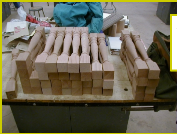
Reproducing balusters from rotted originals
